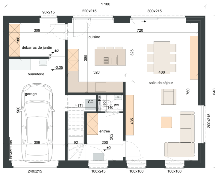
REZ-DE-CHAUSSÉE SURF. = ± 92 m 2
