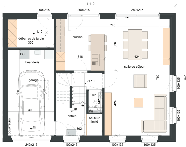
REZ-DE-CHAUSSÉE SURF. = ± 93 m 2
